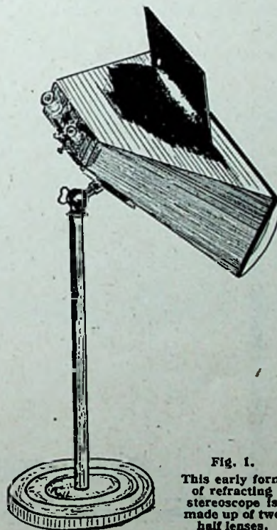
BREWSTER'S LENTICULAR STEREOSCOPE.
